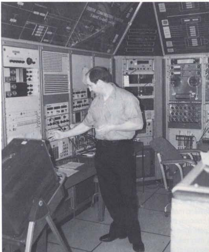
Figure 10 – The bit-error detectors used to establish the overall and link BERs
